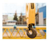
Industrial hoist hooks is one of the most suitable slings in hoisting. It is connected with pulleys to hang on the wire rope of lifting mechanism. And the hook is the most widely usage when lifting cargos. It is made easily and operated practically.
