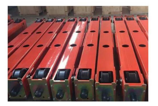
Single Beam End Beam For Bridge Crane is composed by Wheels, motors, buffers, collector base, girder joint plate and bolts, etc. The end beam adopts rectangular control, CNC boring and milling integrated customized machine tool, a one-time completion of opening, boring, drilling. Equipped with high quality reducer, hollow shaft drive, high working level, wide speed adjustment range, widely popular.
