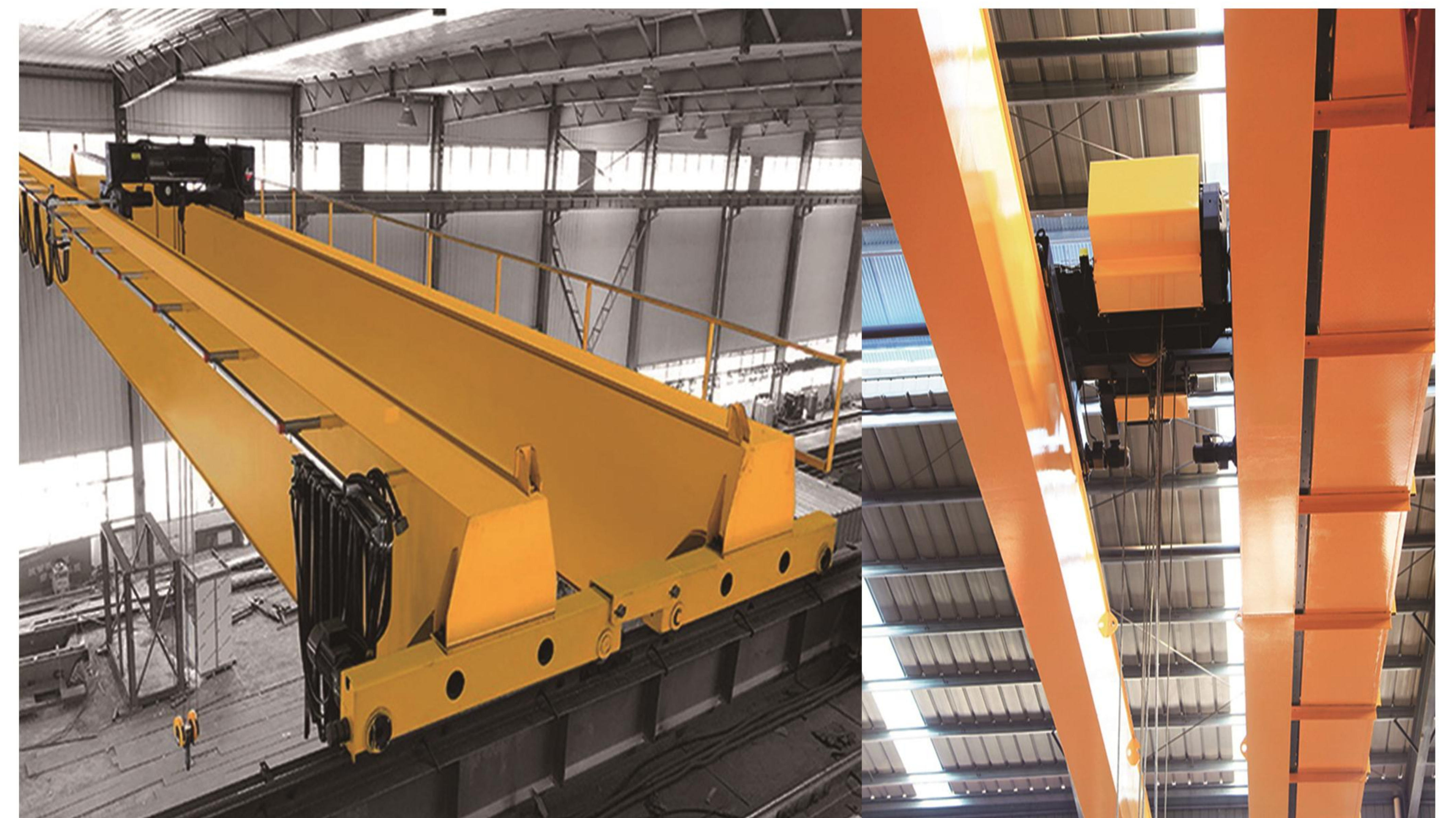
European double girder overhead crane
