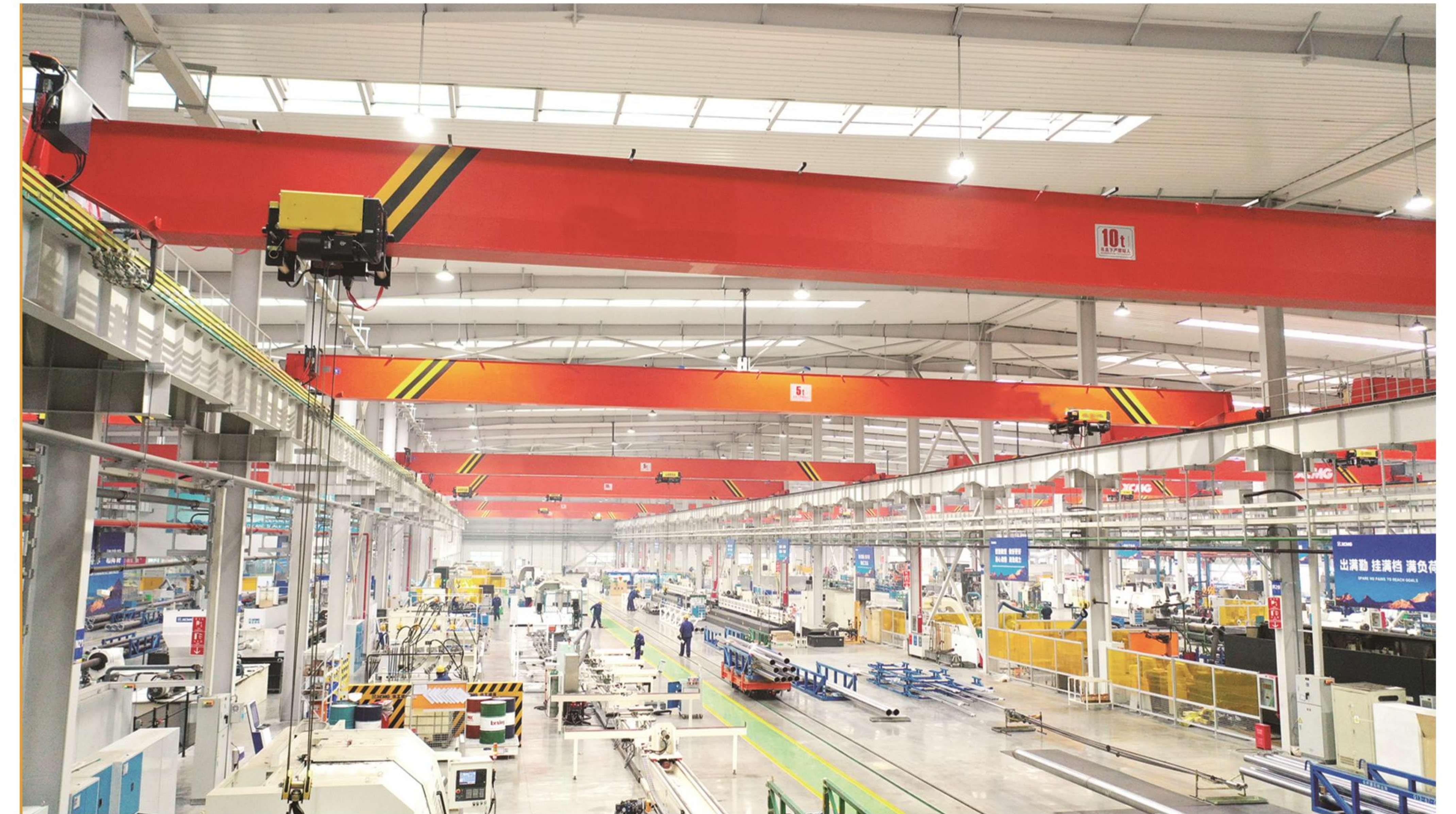
European single girder overhead crane
