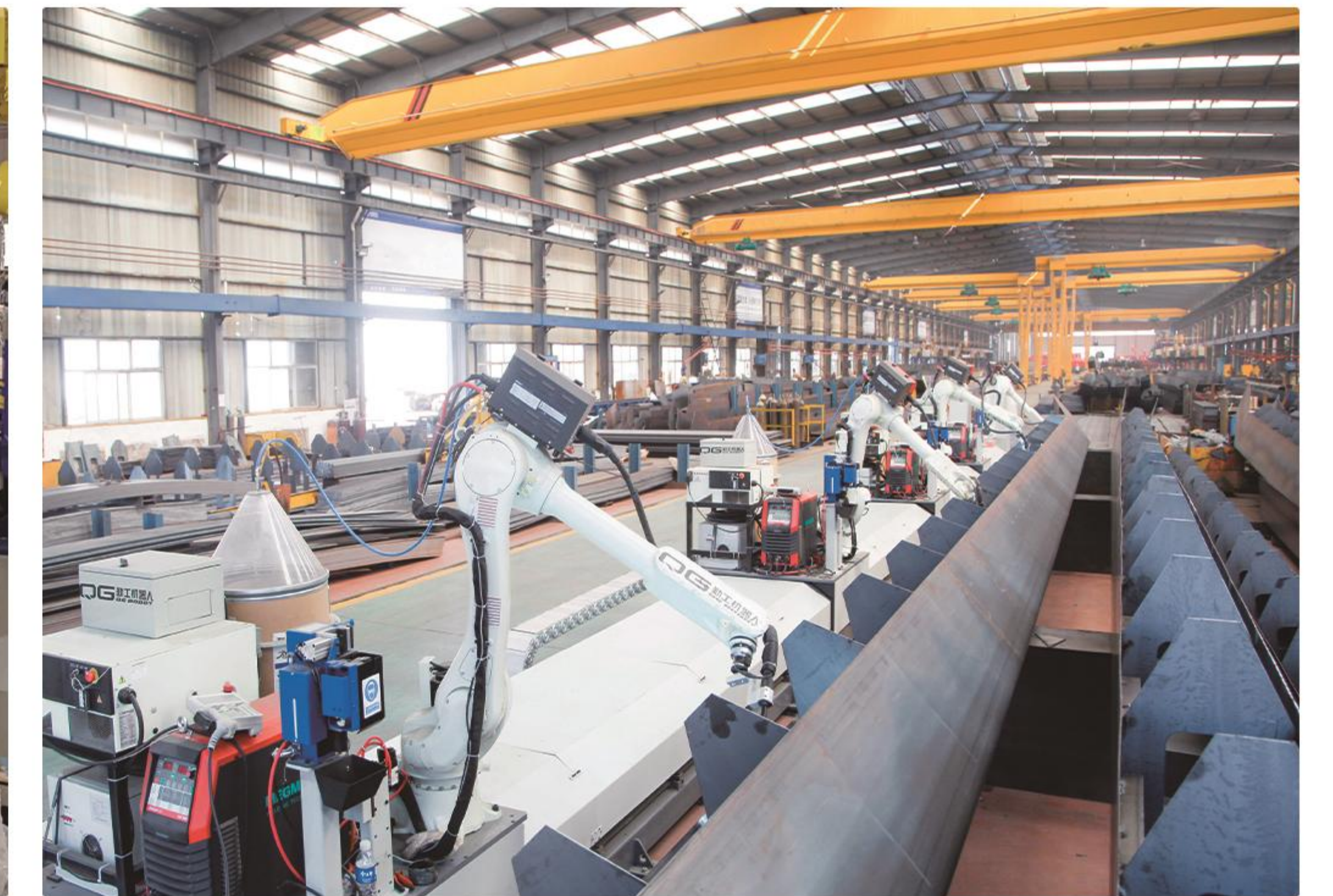
End beam welding robot
