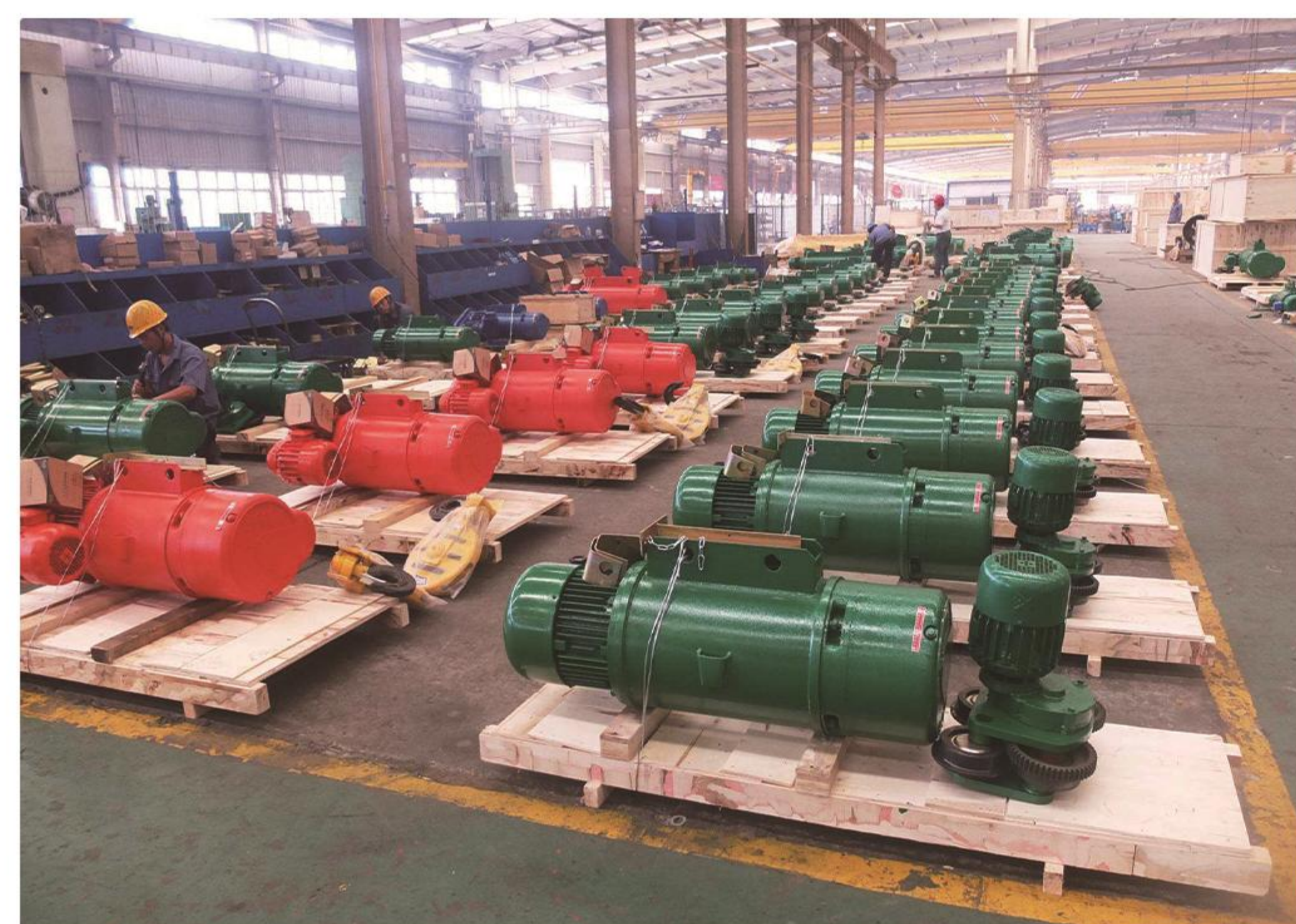
Wire rope electric hoist production workshop
