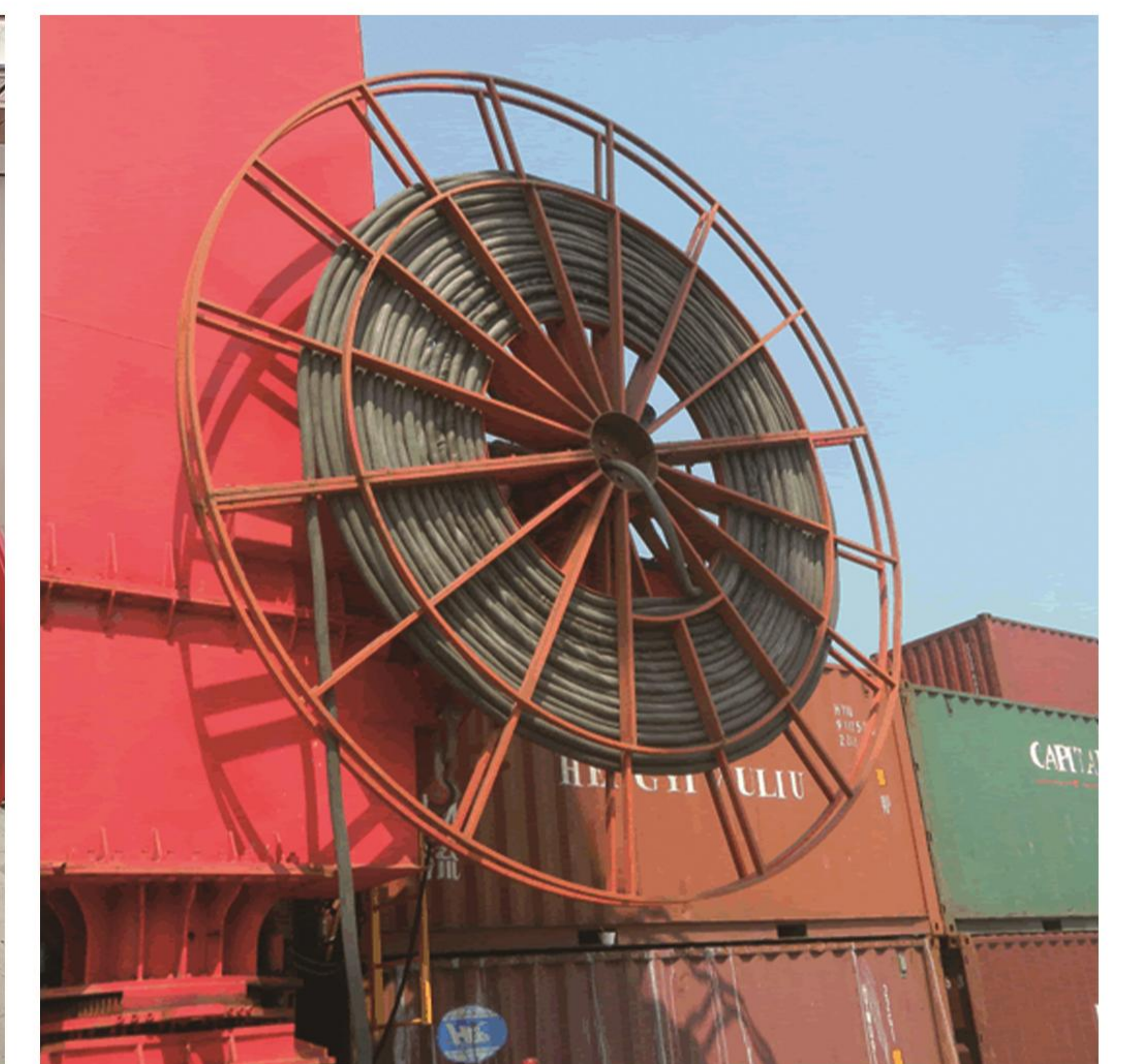
Hydraulic motor type cable reel
