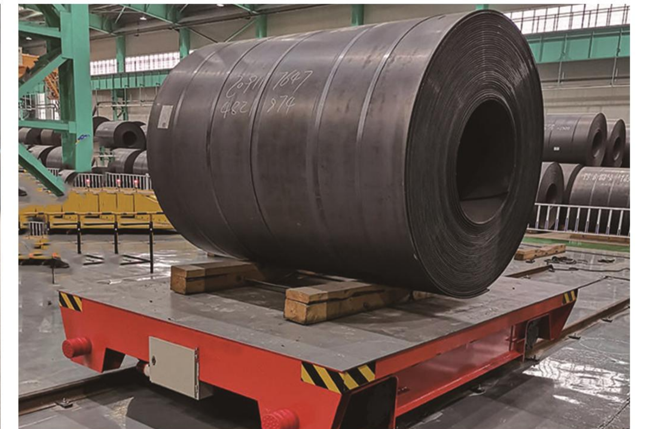
KP cable powered electric flat carts
