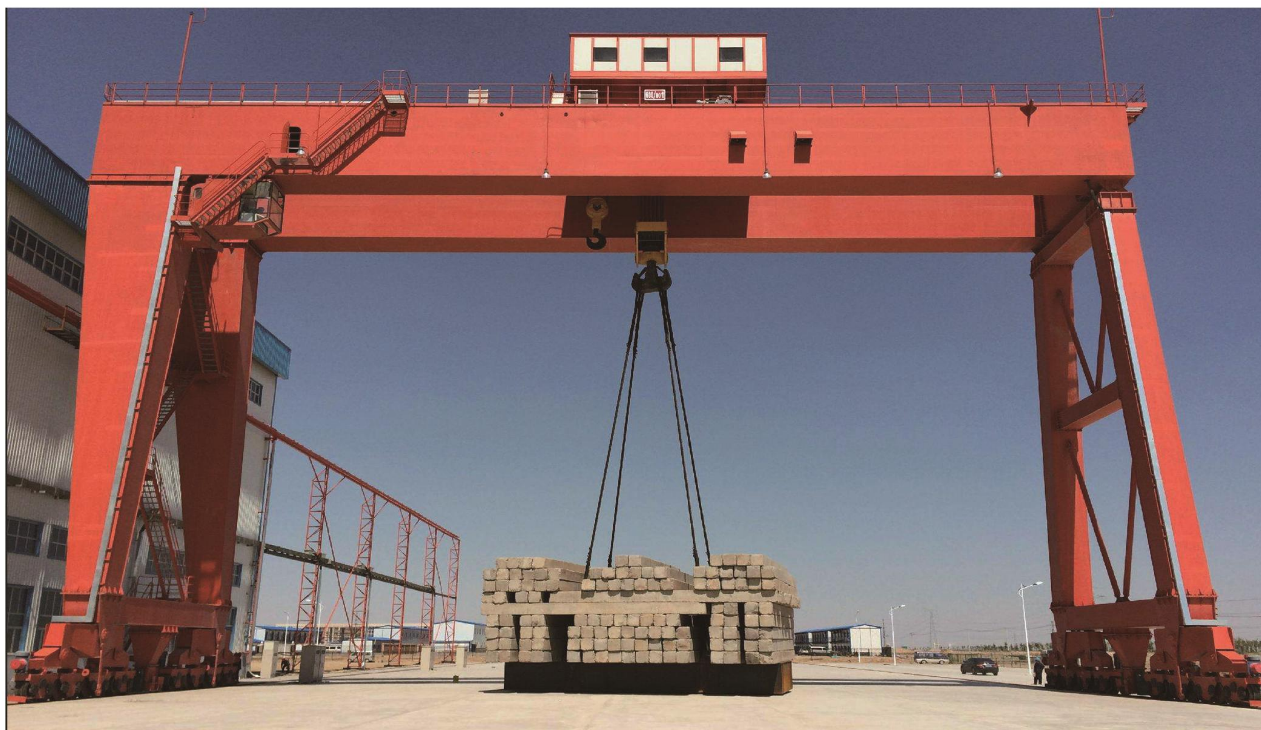
European double beam gantry crane
