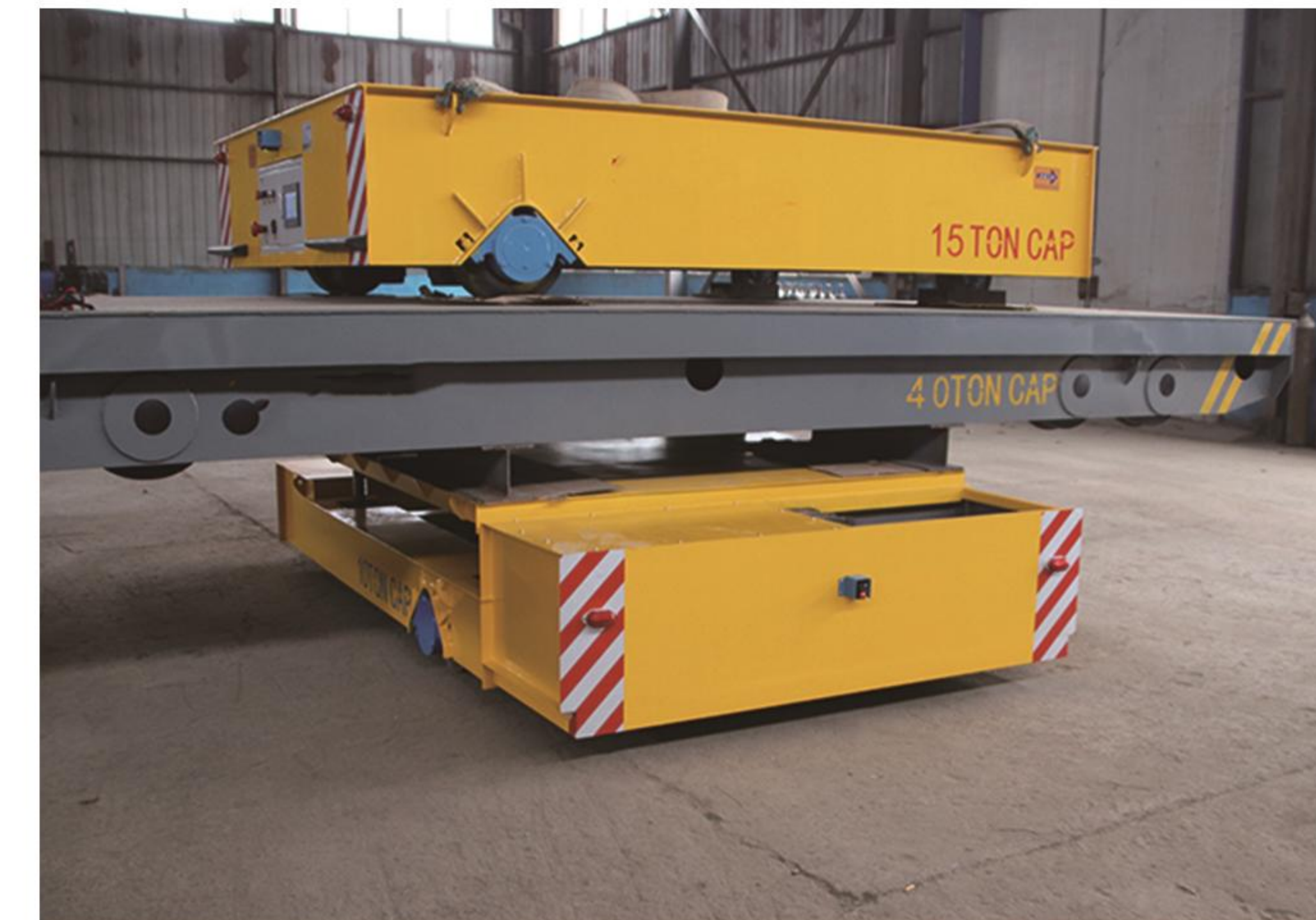
AGV Intelligent trackless electric flat carts
