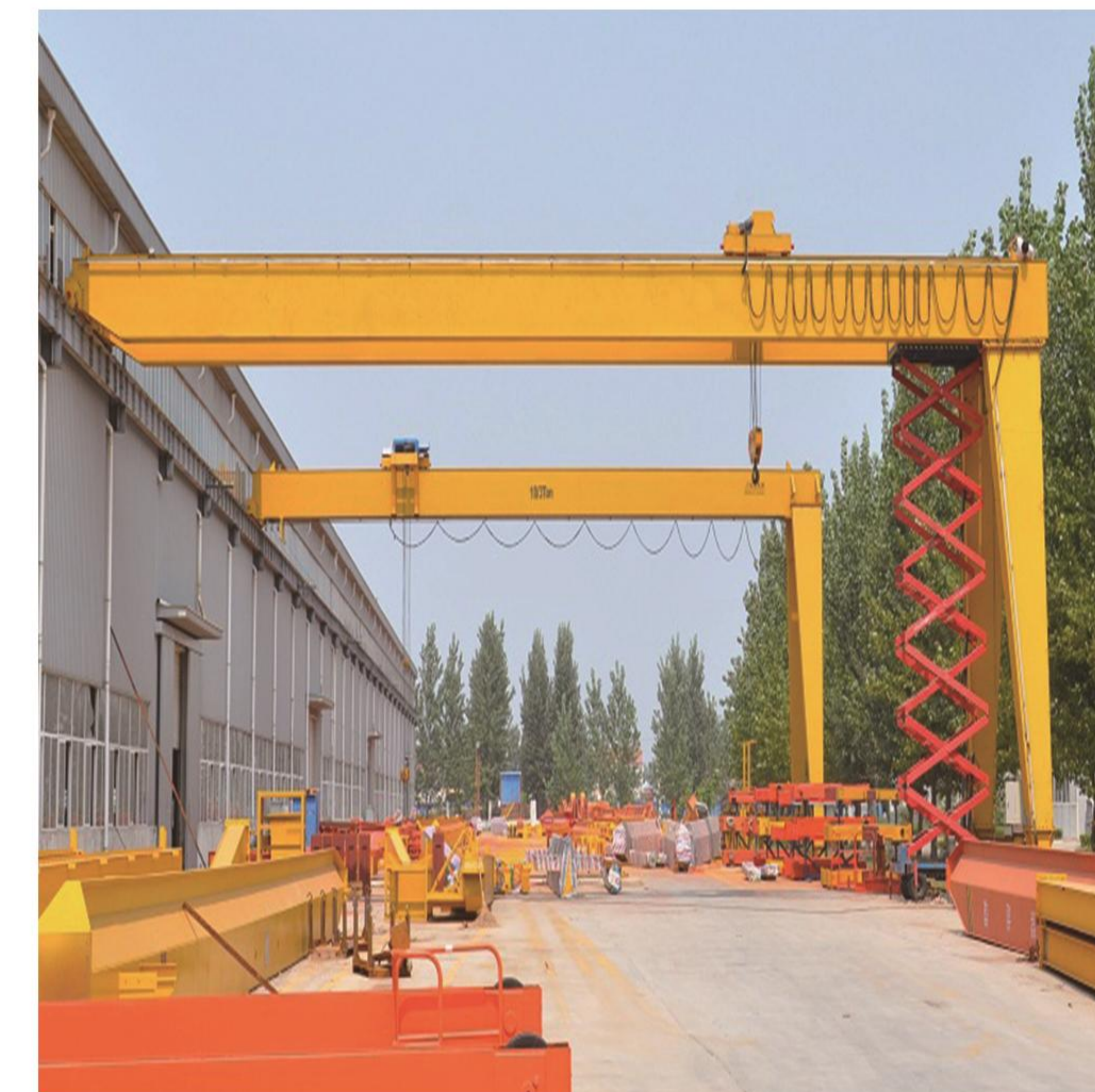
Semi gantry crane
