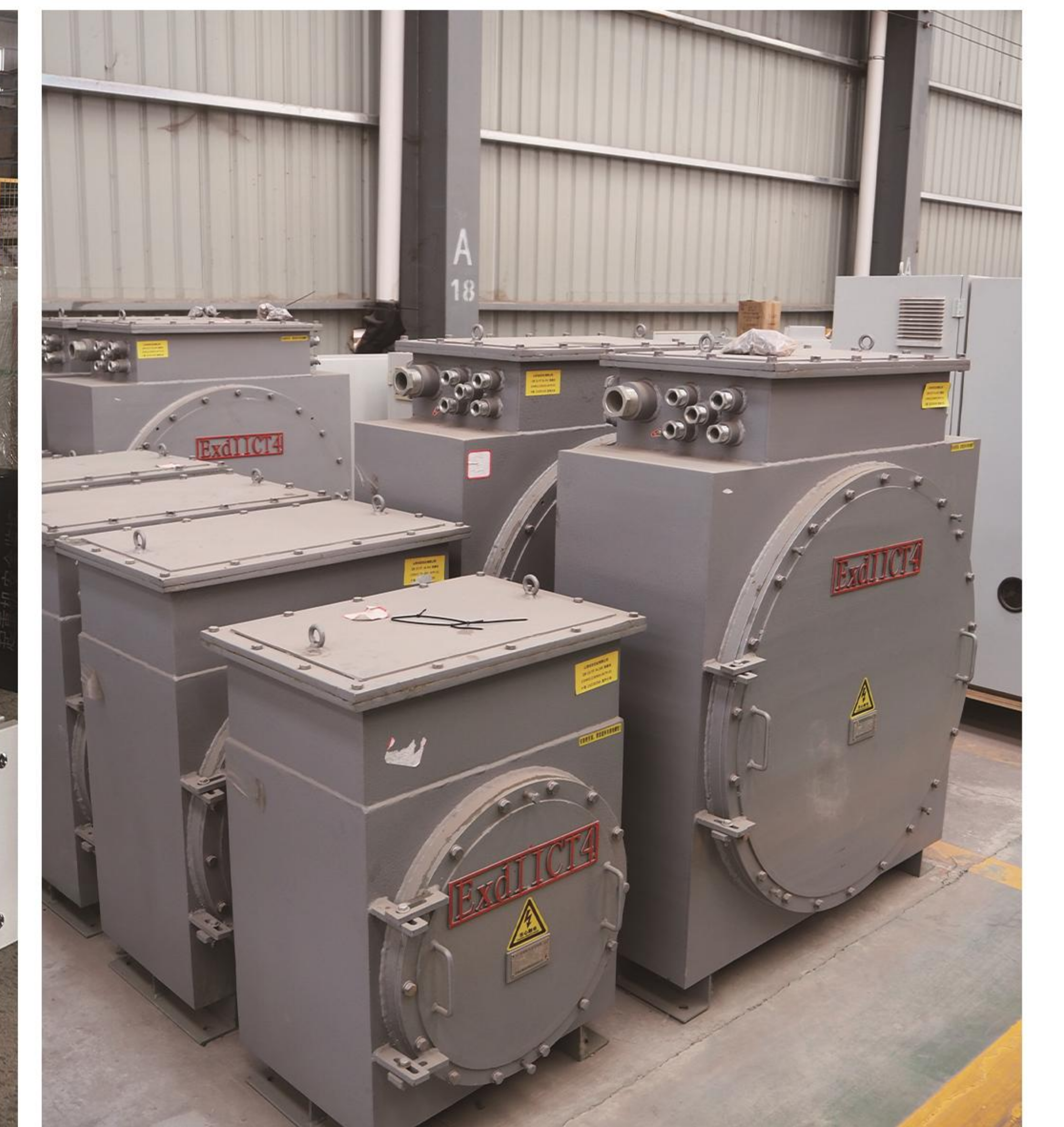
Explosion-proof electrical cabinet
