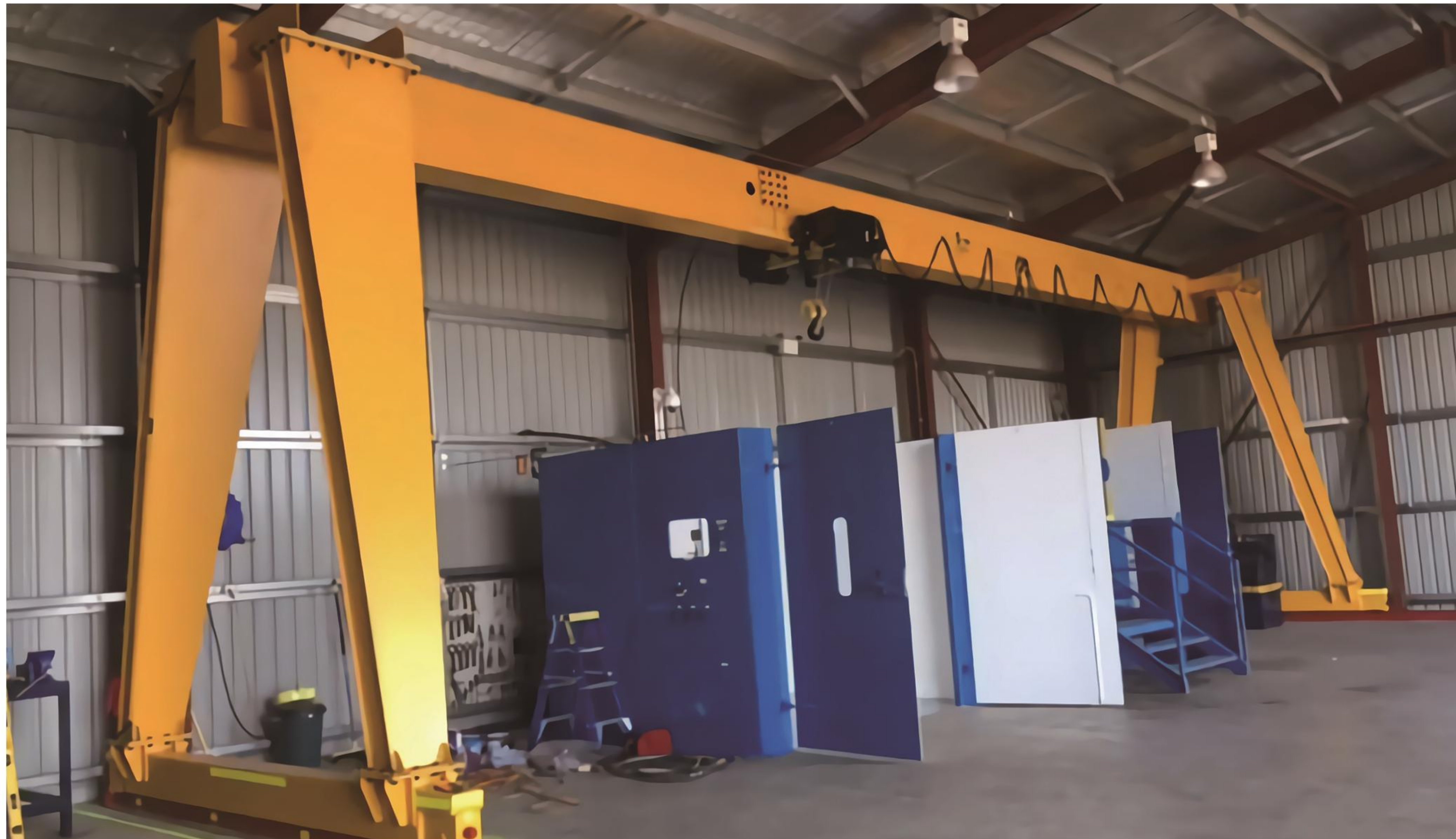
European single beam gantry crane
