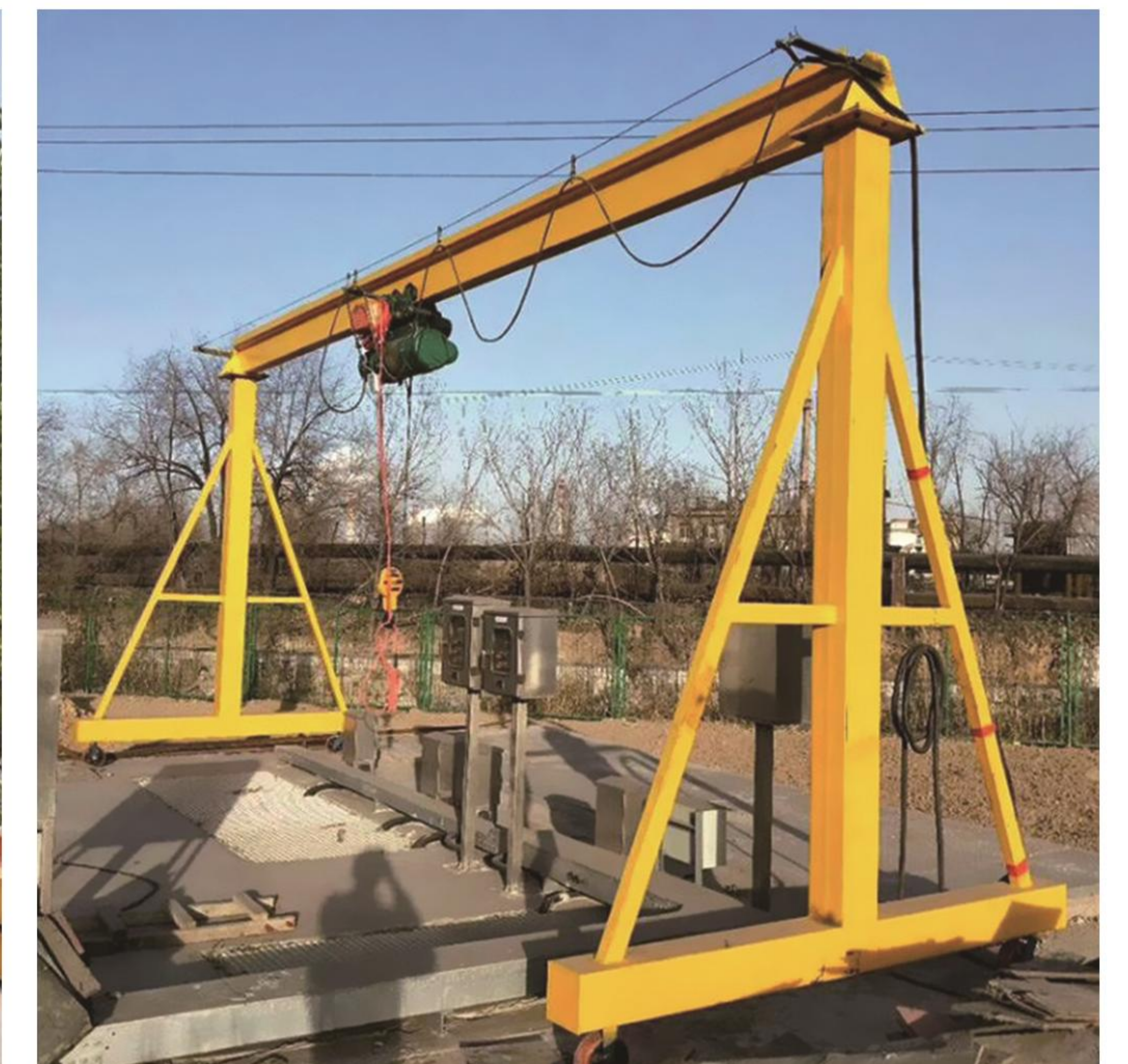
Small gantry crane
