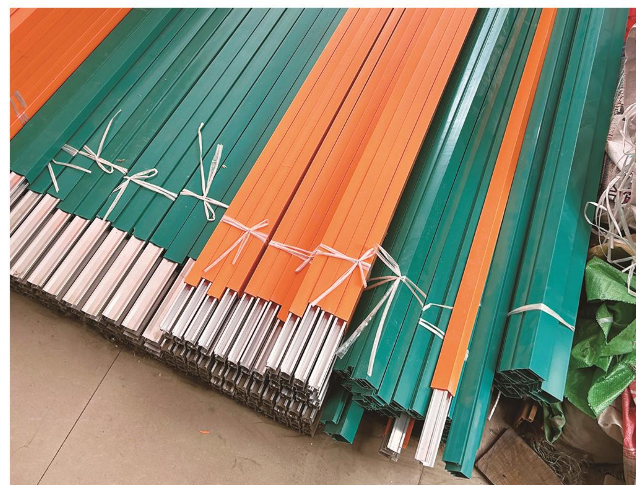
Overhead crane power supply bus bar
