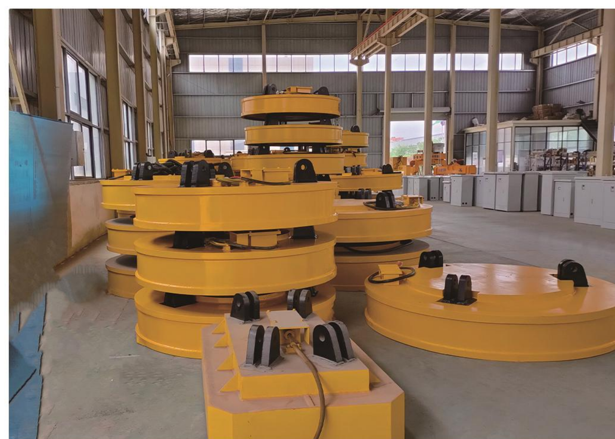
Lifting Electromagnet production workshop
