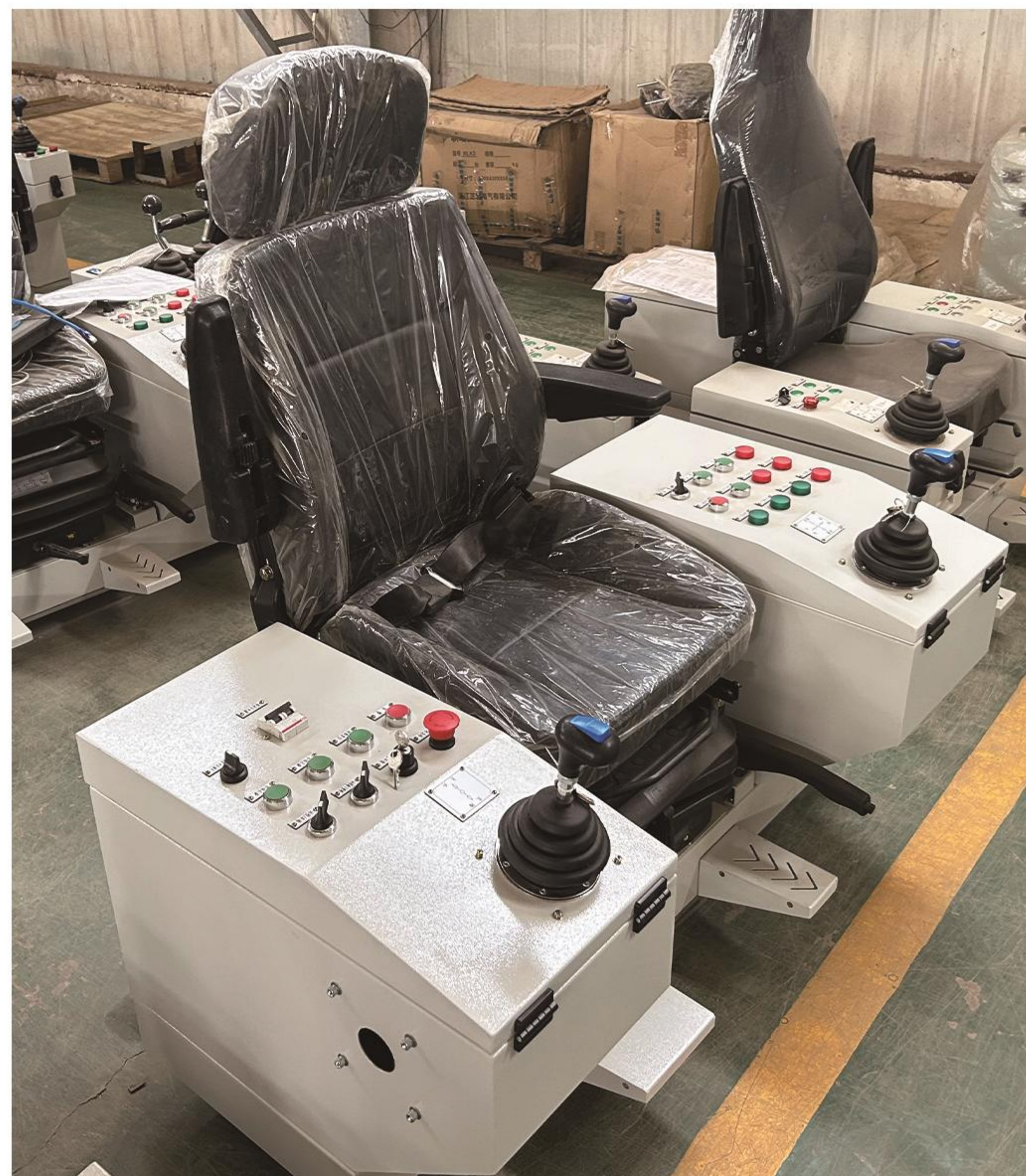
Crane cab controller
